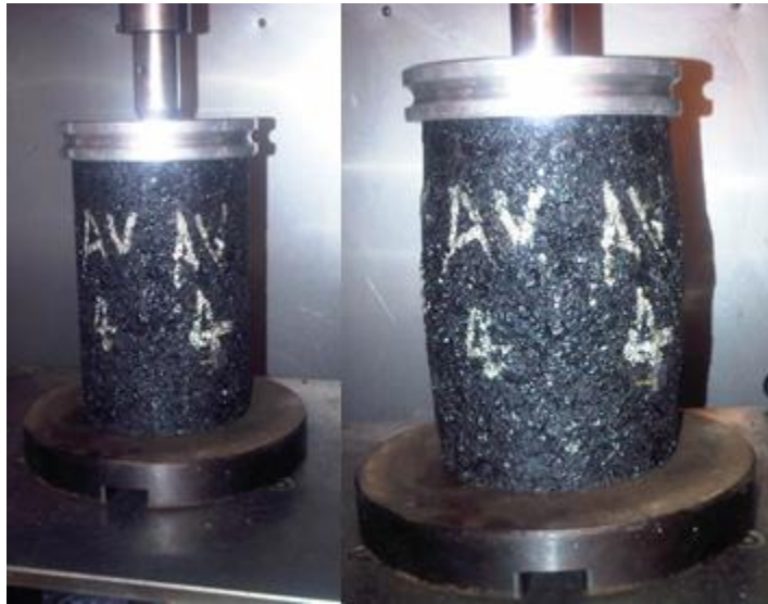
Figure 22. Flow number sample before and after testing
